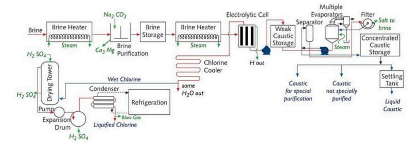
Depending on the end use, chlorine can be compressed at either low-pressure (LP) or high-pressure (HP). In both instances, the chlorine gas can be sent directly to users, or it can be further purified.
