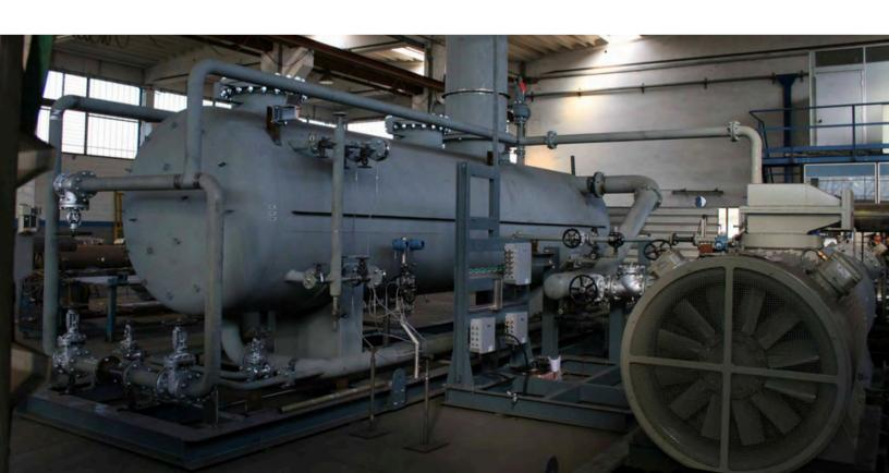
GARO's WAIS is an evolution of traditional FGR systems which exploit the ability of Liquid Ring Compressors to support a wide range of seal liquids. In this way, WAIS can provide a host of benefits over traditional water based seals, particularly in applications where water quality and/or supply are an issue. By using amine as service liquid, Garo's WAIS eliminated the need for a separate gas treating unit, as well as the need for cooling and treatment water. WAIS replaces the
